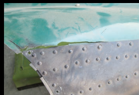
Torn edges in access panels, bad Dzus fasteners, and cracks in the engine cowling all had to be repaired.
