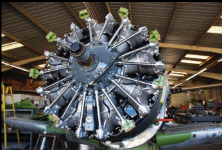
Hanging the freshly overhauled Pratt & Whitney R-985 engine.
