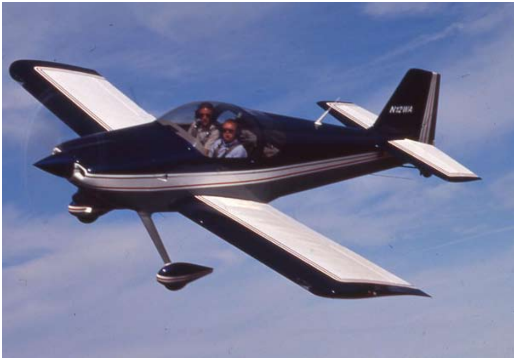
RV-6: There were those who demanded side by side seating... and got it!
