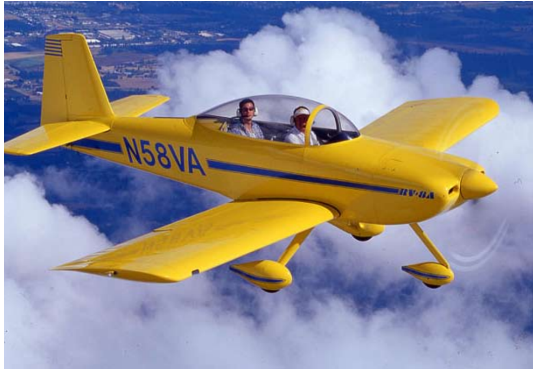
RV-8A: Once again Dick made the move to accommodate those who preferred tricycle landing gear.
