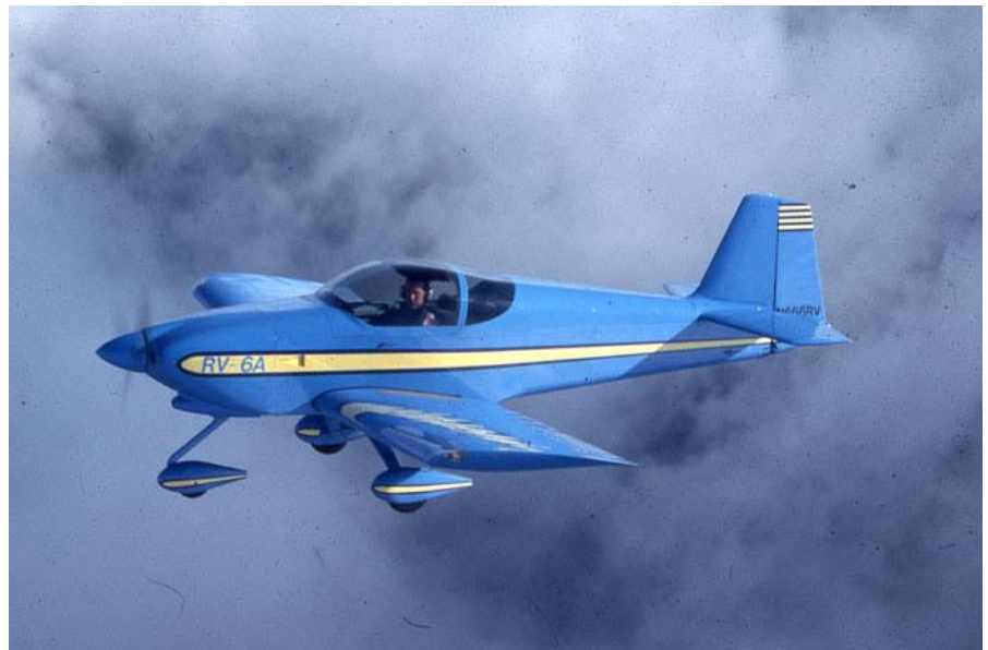
RV-6A: The number of pilots proficient and comfortable in a taildragger was diminishing, so Dick created a tricycle version.
