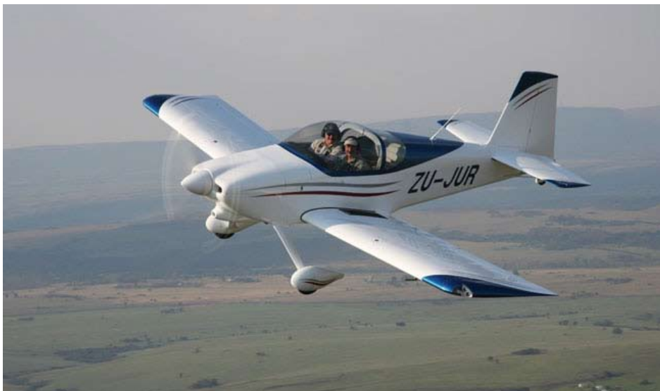
RV-7: This was an upgrade of the RV-6, with an improved kit. It was followed by a Tricycle version, the RV-7A.
