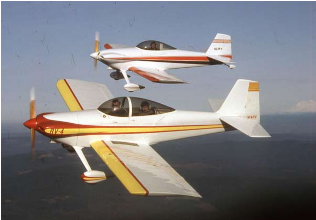
RV-4 and RV-3: After years of appeals, Dick gave the market what it wanted: a two-seat tandem version of the RV-3.
